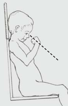
But when the headrest is on the same plane as the back to the wheelchair, it pushes María's head forward. This tilts her head downward making her strain to keep her head lifted. This tension increases her spastic pattern.
