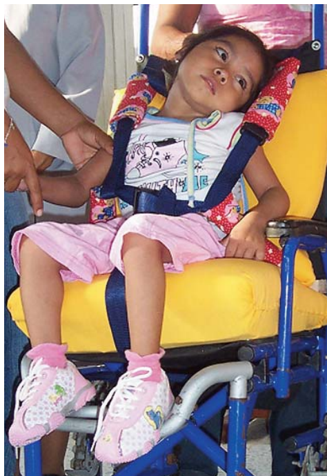
Upholstering the seat before being sure it fit added significantly to the time required to build it, and prevented it from being complete by the end of the workshop.
