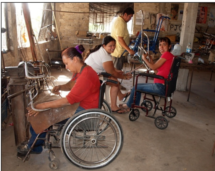
Miguel Angel's aunt (on the right), who has also moved into the Duranguito house with her young daughter, likewise helps in the workshop. Here she, Yasmín and Carmin (foreground) use strips of emory paper to sand the rust off the metal tubes (electrical pipe) of the frames of the wheelchairs.
