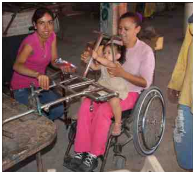
Miguel Angel's aunt (on the right), who has also moved into the Duranguito house with her young daughter, likewise helps in the workshop. Here she, Yasmín and Carmin (foreground) use strips of emory paper to sand the rust off the metal tubes (electrical pipe) of the frames of the wheelchairs.
