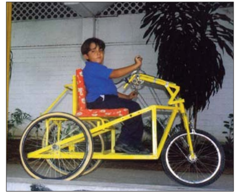
A manual tricycle was made for this child with spina bifida, who rides a long way to school on uneven roads. Tricycles are faster and safer than normal wheelchairs.
