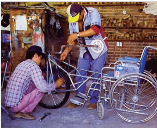
For this reason, the Duranguito team has experimented with a collapsible tricycle, where the front part with the large wheel can be instantly removed—so that the rider can enter buildings with the back part, which is essentially a regular wheelchair.
