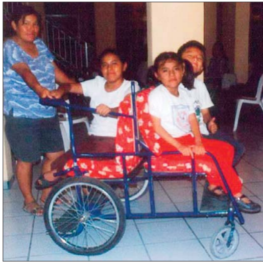
At the mother's request, the team made a pushcart with 4 seats, so that she could move her children about more easily. They included the fourth seat to accommodate yet another child, since the mother at the time was pregnant. (They also offered her advice on family planning.)
