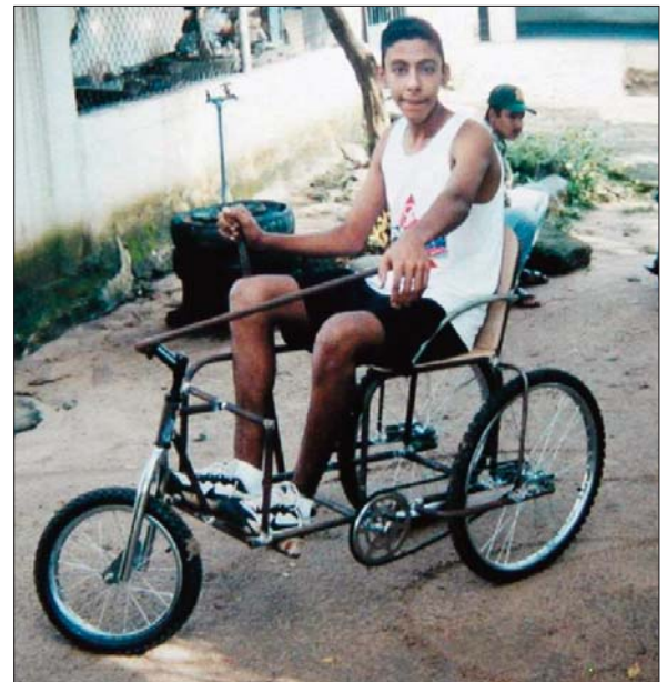
For people who have difficulty walking, or use crutches, a hand-powered tricycle is convenient for going long distances. But for someone who can't walk at all, the large size of the tricycle is a disadvantage, particularly inside of buildings.
