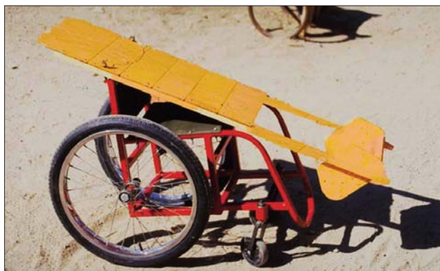
The inclined gurney is mounted on a wheelchair.
