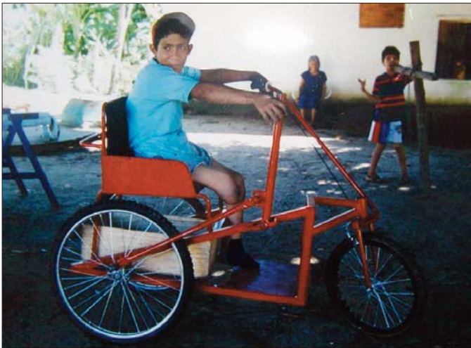
An alternative tricycle design is powered with a large hand lever. The rider pumps the lever with one hand while steering with the other. This design is especially useful for a hemiplegic person, or anyone with one hand that is weaker.
