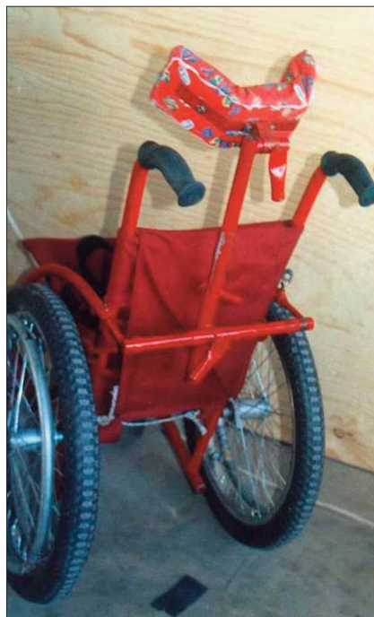
The headrest of this chair is fully adjustable in terms of height, angle of recline, lateral pivot, and up-or-down tilt.
