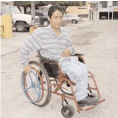
Figure 1 - The one-hand-drive wheelchair has handrims for both wheels on one side.
