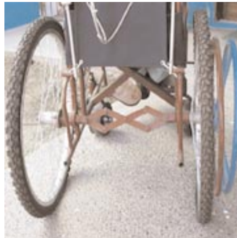
Figure 2 - This innovative wheelchair has a folding axle to transfer power from one hand rim to the far side.
