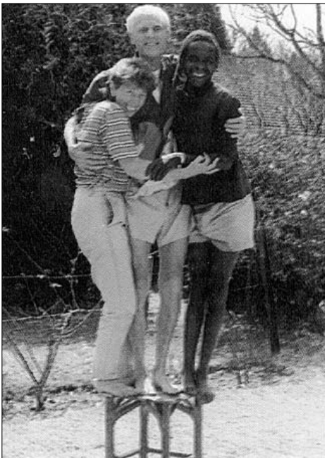
This stool, made only of paper and cardboard, can support 3 people. (Photo from APT manual by Bevill Packer.)
